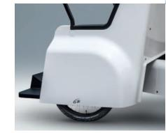
Lotta is a high-class urban vehicle. Its body is made of light and durable polyester and glass fibre laminate.
